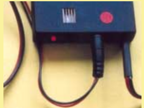
The two batteries with the associated mains PSU for charging (picture at top of right-hand page). Next to the red dot can be seen the silver-coloured heat-sink for the charger electronics. When the battery is connected to the mains PSU, the red LED adjacent to the charge plug glows to indicate that charging is taking place (picture above).
